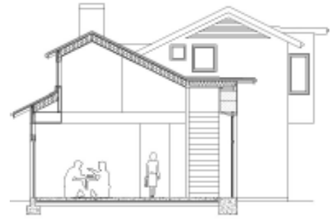
South-facing clerestory windows ensure solar energy is absorbed by plaster walls
